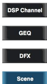
Touch anyone of these controls, the corresponding background will illuminate, you can load preset of selected controls.
