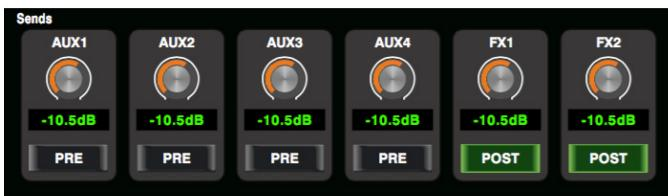
Touch PRE on the screen, it will switch to POST, the AUX & FX send will derive its signals from all channels post-fader. If the icon has not been pressed and not illuminate, by default, the AUX & FX Send will derive its signal from all channels pre-fader and all unaffected by the sending channel's fader position. In a word, touch PRE and switch it to POST, then you can adjust its level by sliding fader. Otherwise, the fader wouldn't function on level adjustment.
