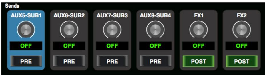
Touch AUX5-8(SUB1-4) and FX1-2 on the LCD screen to assign input channel audio to these channels or buses. To adjust output level of the channel audio, you can rotate Parameter Adjust knob on the panel. For other icon functions in this page, they are the same with those in SUB1-4 mode.
