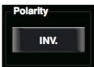
Touch it in Polarity to invert the phase of the selected channel's signal (to alter the phase by 180°). If the phase reverse is active the button will illuminate. The LCD display shows the phase reverse setting in real time. The Polarity control can be used to correct audio signals which are out of phase as well as to cancel/reinforce each other.
