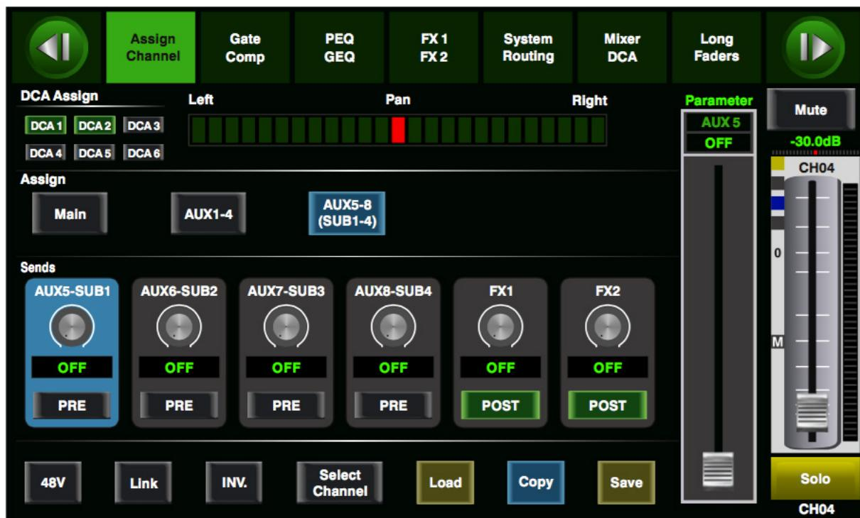
When switch Sub1-4 mode to AUX 5-8 mode, the corresponding page is as below picture show, this function enable output assignments to be more.
